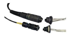
Delphi™ branded Hermaphroditic Connectors have been developed to meet the stringent demands of outdoor applications and to provide superior optical performance. Hermaphroditic Connectors allow concatenations (linked together in series) of cable assemblies to extend equipment separation without concern for connector male / female interface compatibility. Additionally "blind mating" and "scoopproof" features help ensure easy to mate interconnects.
